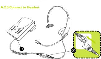
The A10 Alpha provides the choice of using telephone headset (with RI-11 Modular Plug) or stereo computer headset (with 3.5mm Diameter Plugs) according to your preference.
